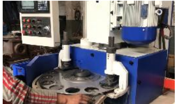
DUPLEX GRINDING MACHINE
